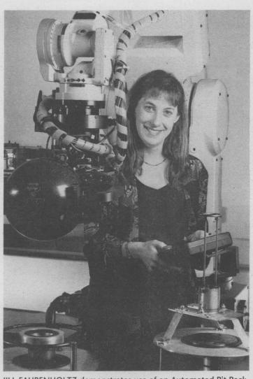
JILL FAHRENHOLTZ demonstrates use of an Automated Pit Packaging system developed at Sandia and delivered to Pantex. The bowling ball approximates the size and weight of a nuclear weapon "pit."
